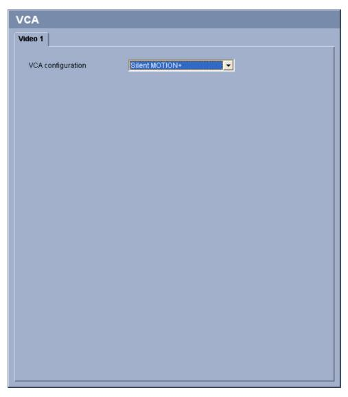
The VideoJet X10 contains an integrated video content analysis (VCA), which can detect and analyze changes in the signal on the basis of image processing. Such changes can be due to movements in the camera's field of view.
